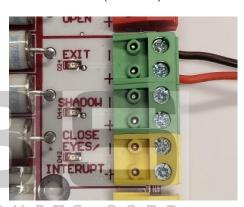
\*Picture to give an example to how to run the attached connector wires from the detector to the main control board.
